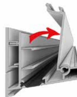
7 Insert ringbeam flaps by locating hinge part of the flap into the main ringbeam at approx 80 degrees as shown.
