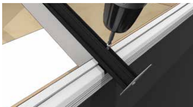
15 Check that the rafter is square to the ringbeam. Fix the 4.8 x 50mm screw supplied centrally through the bottom of the transom rafter as shown to secure the rafter.
