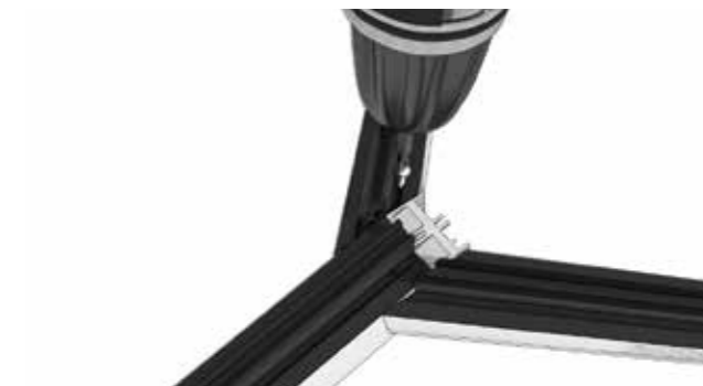
10 Tighten pre-fixed screw at the top of the hip rafter to hold bracket.
