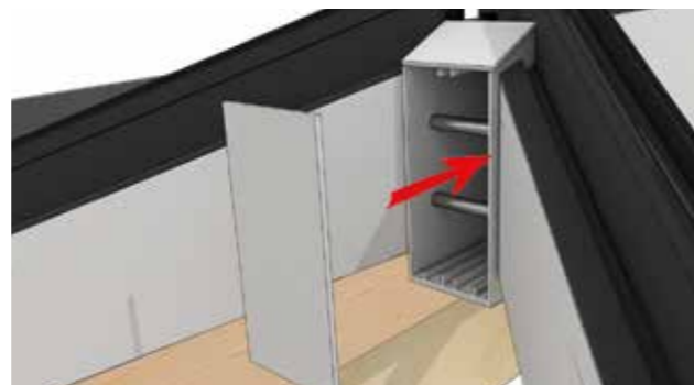
16 Using a small bead of sealant, apply to the rear of the ridge end closer plate and secure to the cut end of the ridge as shown.
