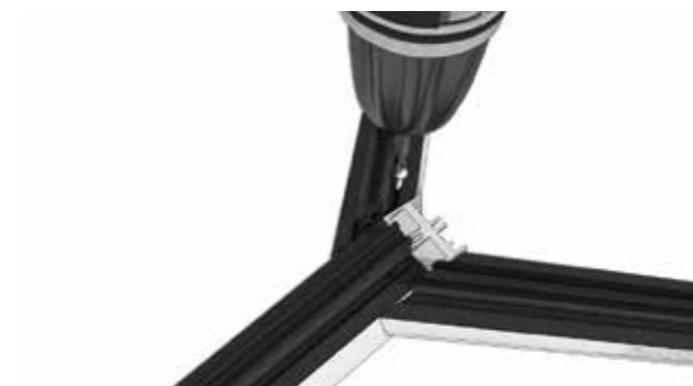
9 Push the joint tight against the ridge and fix down through the rafter with the supplied screw approximately 25mm from the top with a 4.2 x 25mm screw. Repeat on the opposite side.
