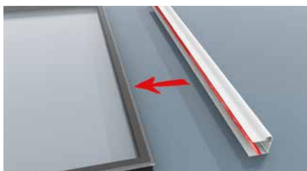
17 Apply a bead of sealant to glazing end closer and fit centrally to glass units.
