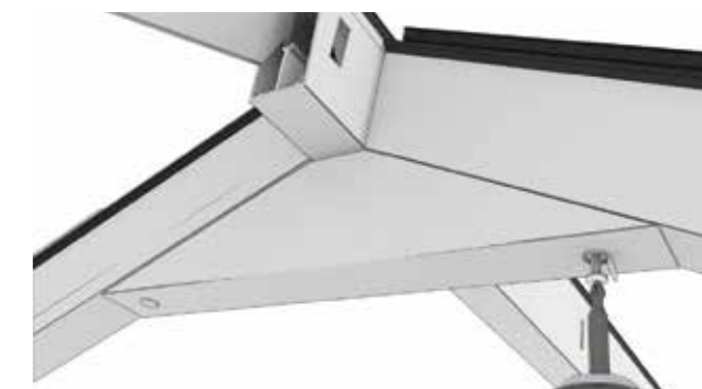
8 Secure in pre-drilled holes with supplied 5 x 70mm screws and fit cap covers.
